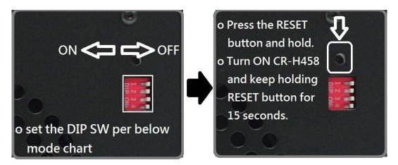
DIP switch code(from left to right) "DIP switch 1", "DIP switch 2" and "DIP switch 3" "DIP switch 4".
