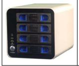
4. Slide the installed trays back to the enclosure, a click sound is heard to confirm the tray is locked in the enclosure. Then connect the eSATA or USB 3.0 cable and turn ON the device
