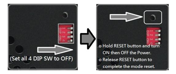
B. To set the DIP switch to a new RAID mode, please follow the mode chart as below, press the RESET button and hold it, turn on the box and keep hold reset button for 15sec.
