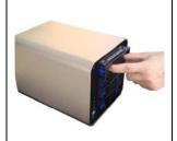
Press 2 blue door latches inward to release the tray lock, then pull out the tray.
