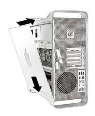
8. Insert side panel and close the latch Slide side panel down and toward case. Close latch and reconnect the external cables and the power cord.
