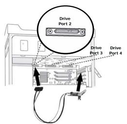
5. Install the Areca ARC-5020-3 Card The ARC-5020-3 has a cable and a card end. Install the cable end into Drive Port 2 on the motherboard. Then slide the card end into the slot where the PCI bracket was removed. Make sure the cable connector is securely into the SATA port on the motherboard and the card is fully seated into the slot.
